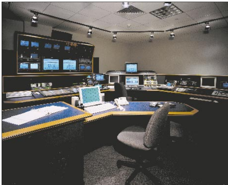
The majority of the programming the station takes in is ready to air, but customization and preparation is often needed. Pictured is one of the two main linear online editing rooms, utilizing a GVG Kalypso two-M/E production switcher and an Accom Axial 3000 online editing system.
