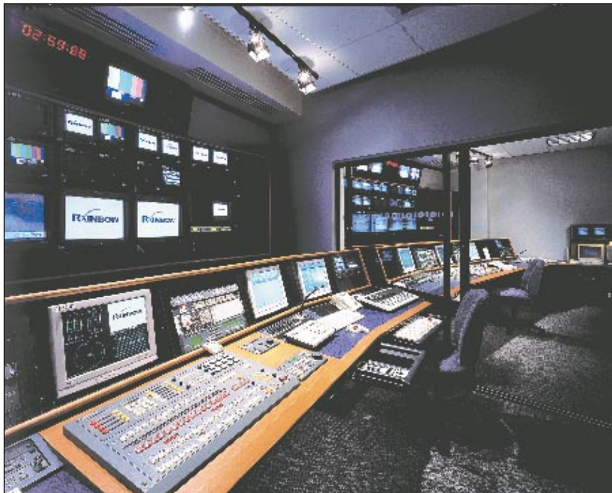
RNC created flexible "clusters" of multichannel control rooms to allow switching between individualized live programming and control of up to four channels in multichannel mode. The single-tier control room above includes a GVG M2100 master control switcher, GVG Profile XP servers, and Sony monitors and VTRs.
